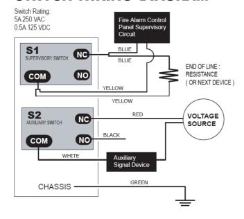
The diagram shows a typical connection between the common terminal and the normally closed terminal. The indicator light and alarm will stay on until the valve is fully open. When the valve is fully open, the indicator light and alarm will go out.
